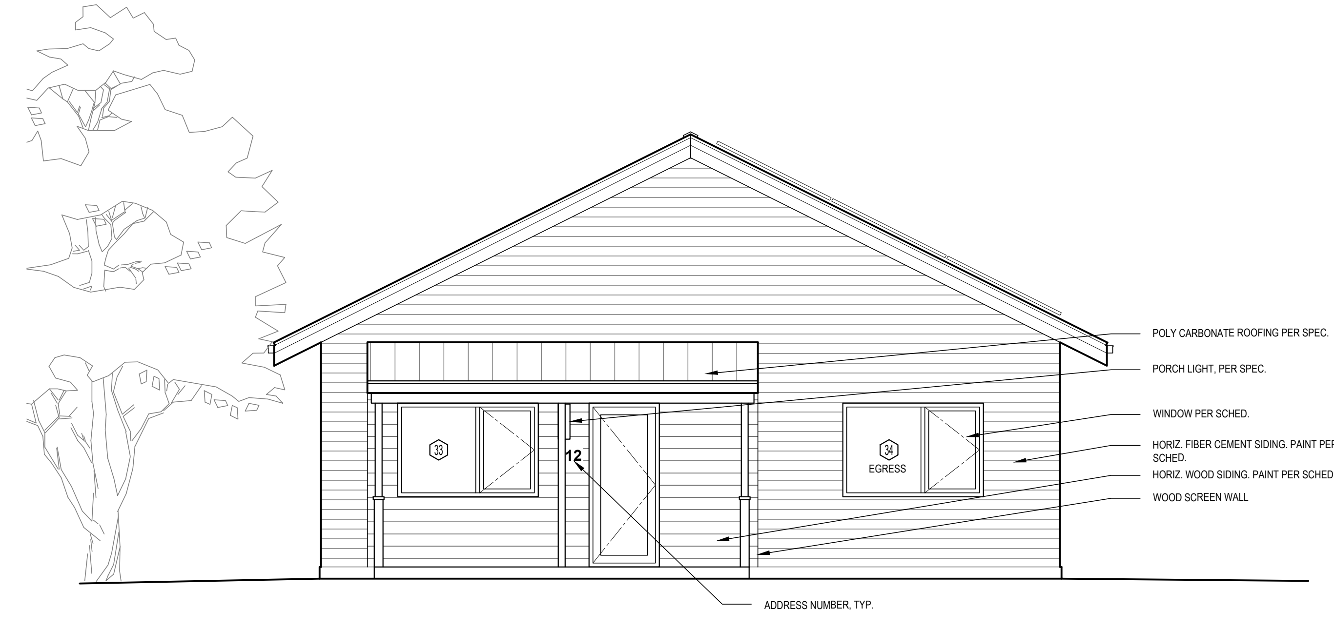
2 SOUTH ELEVATION ADA Scale: 1/4"=1'-0"
